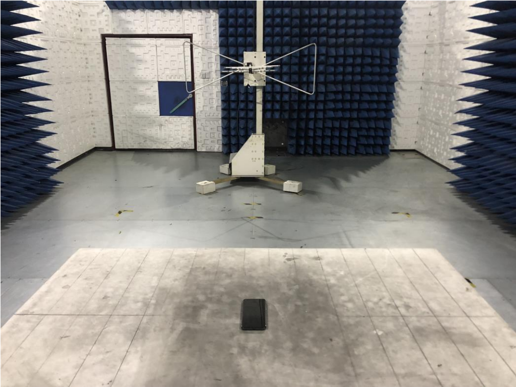
FCC RADIATED EMISSION TEST SETUP BELOW 1GHZ
