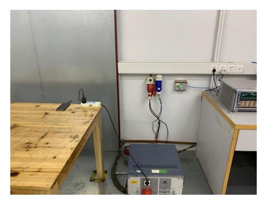
FCC RADIATED EMISSION TEST SETUP BELOW 1GHZ
