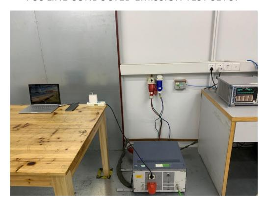
FCC RADIATED EMISSION TEST SETUP
