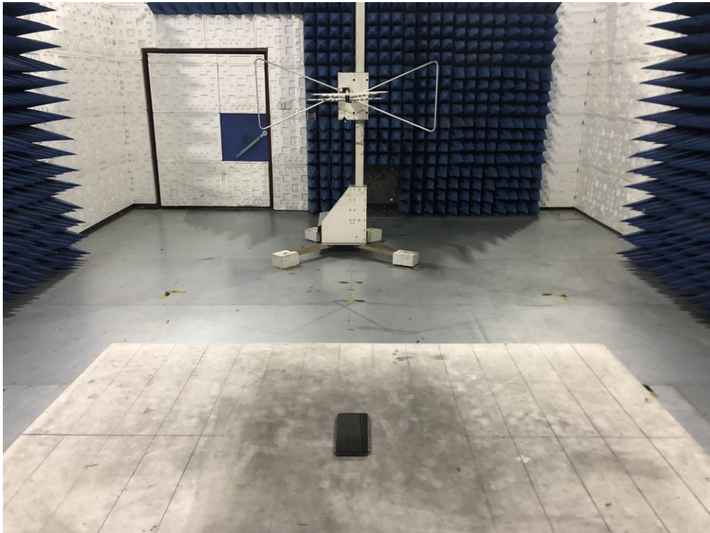
RADIATED EMISSION TEST SETUP ABOVE 1GHZ
