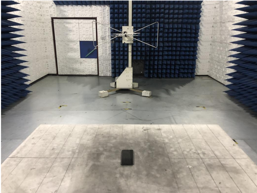
RADIATED EMISSION TEST SETUP ABOVE 1GHZ
