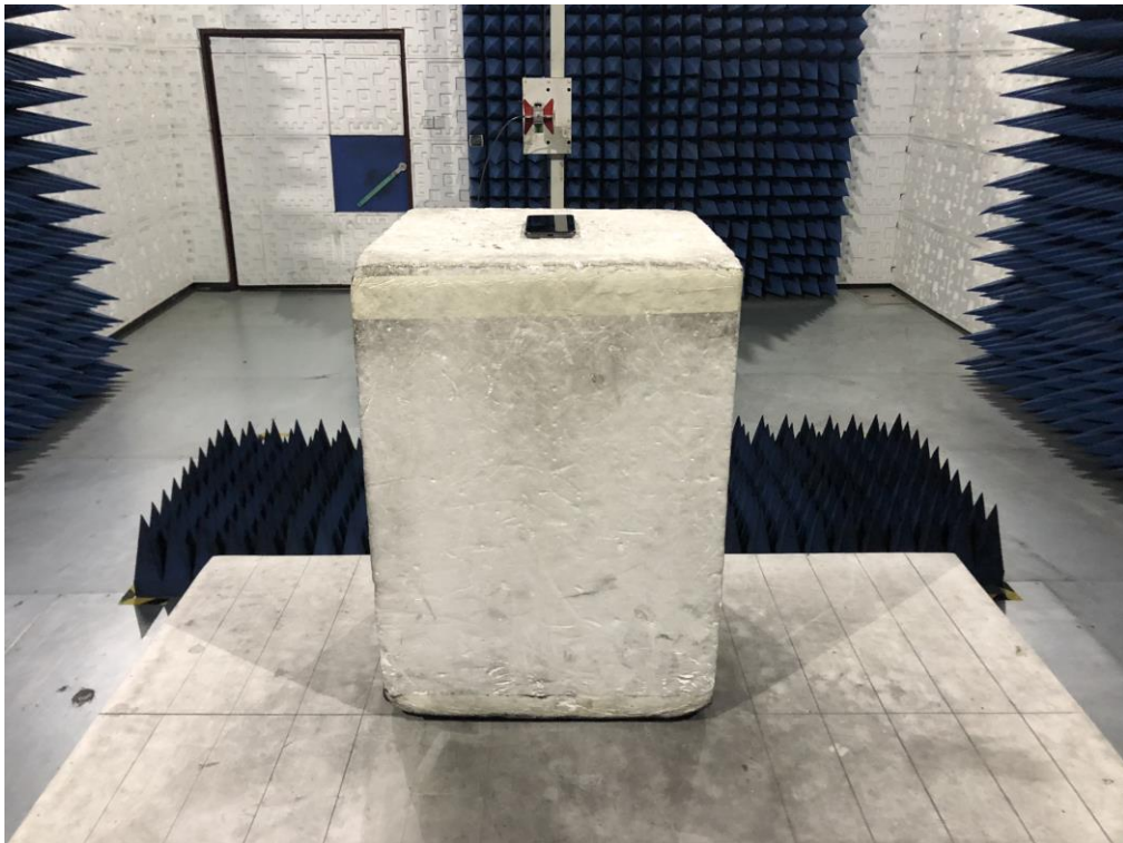
RADIATED EMISSION TEST SETUP ABOVE 1GHZ
