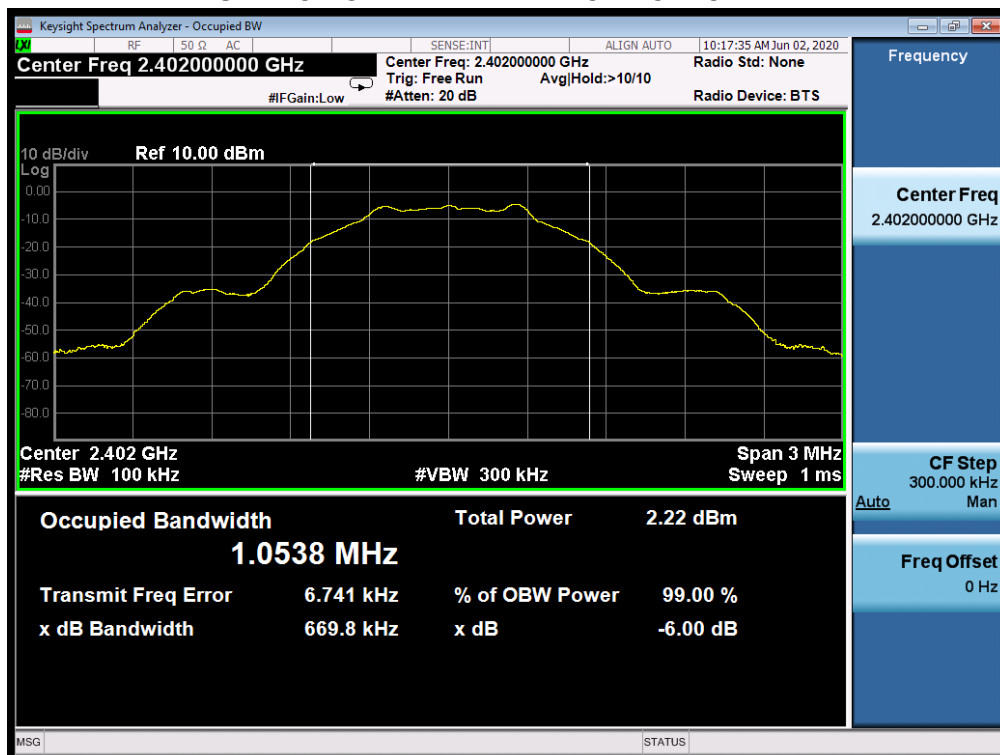
TEST PLOT OF BANDWIDTH FOR LOW CHANNEL
