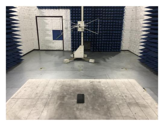
RADIATED EMISSION TEST SETUP ABOVE 1GHZ
