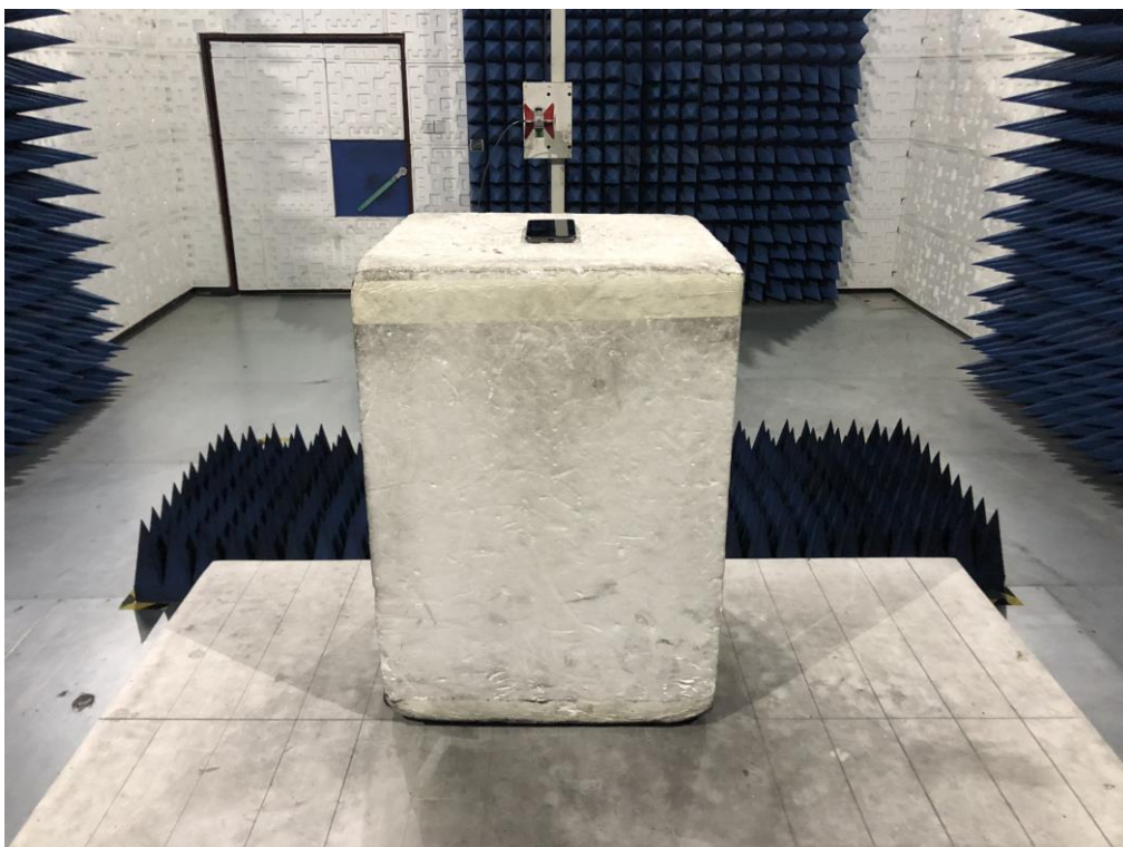
RADIATED EMISSION TEST SETUP ABOVE 1GHZ
