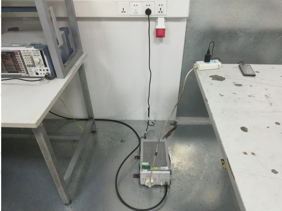
Photo of Conducted Emission Measurement
