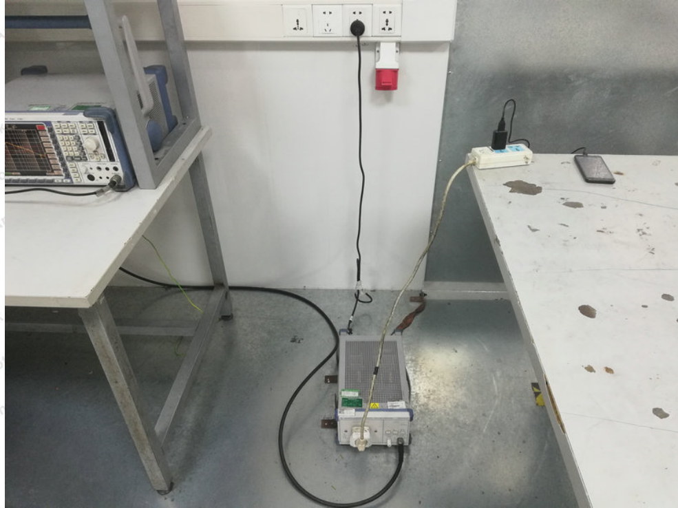
Photo of Conducted Emission Measurement
