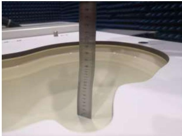
Fig. 9.7 Photo of Liquid Height for Head SAR
