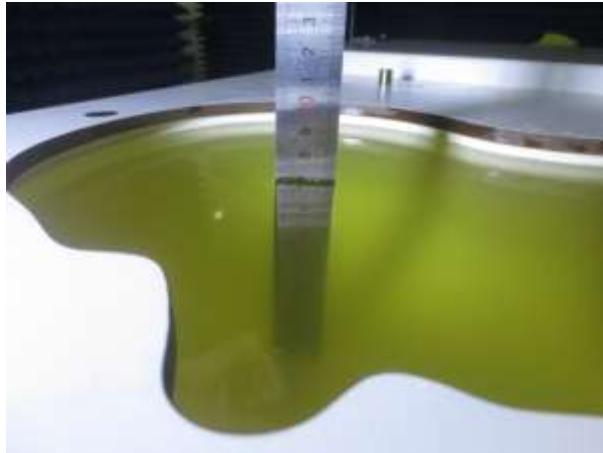
Fig. 9.1 Photo of Liquid Height for Head SAR
