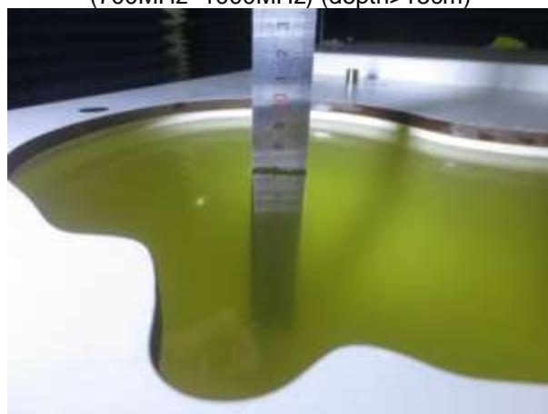
Fig. 9.3 Photo of Liquid Height for Head SAR
