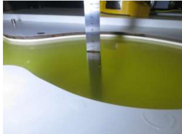
Fig. 9.2 Photo of Liquid Height for Body SAR
