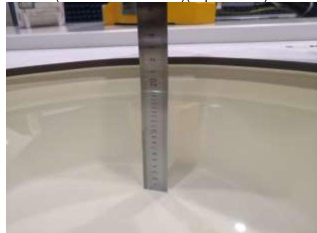
Fig. 9.8 Photo of Liquid Height for Body SAR of Twin
