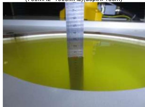
Fig. 9.4 Photo of Liquid Height for Body SAR
