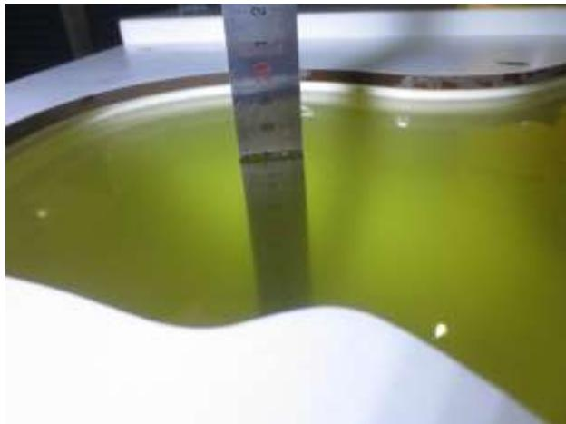
Fig. 9.5 Photo of Liquid Height for Head SAR
