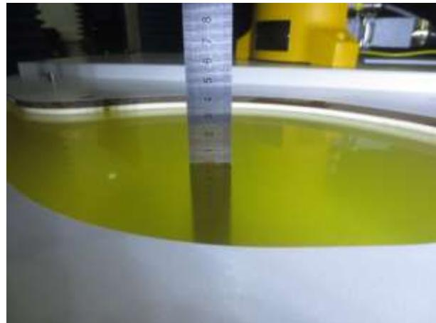
Fig. 9.6 Photo of Liquid Height for Body SAR
