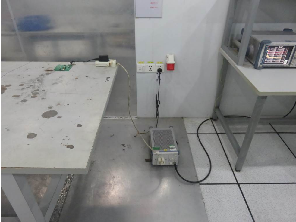
Photo of Conducted Emission Measurement
