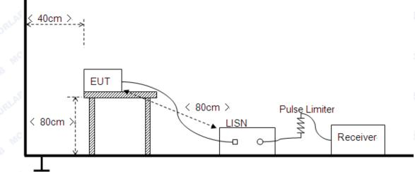
The EUT is placed on a 0.8m high insulating table, which stands on the grounded conducting floor, and keeps 0.4m away from the grounded conducting wall. The EUT is connected to the power mains through a LISN which provides  $50\Omega/50\mu$ H of coupling impedance for the measuring instrument. A Pulse Limiter is used to protect the measuring instrument. The factors of the whole test system are calibrated to correct the reading.
