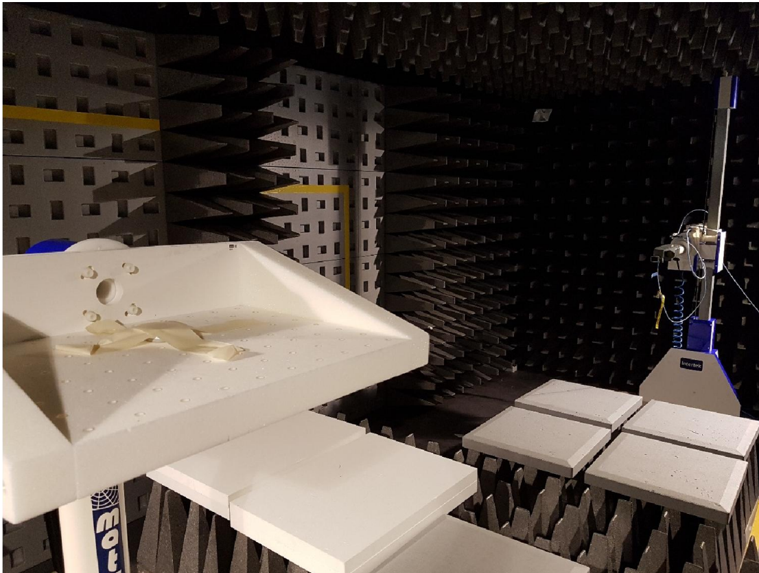
Test set up radiated emission 18 GHz – 26.5 GHz
