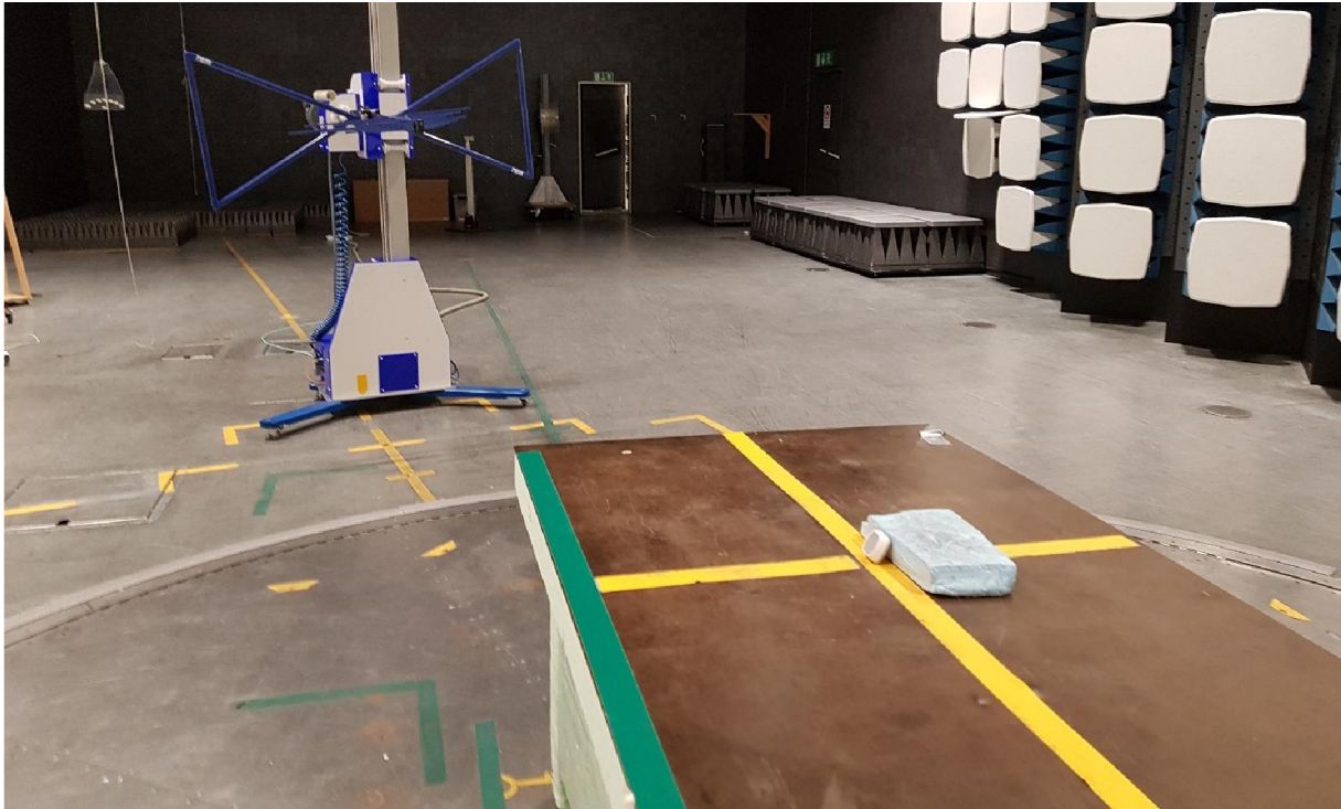
Test set up radiated emission 30 MHz – 1GHz
