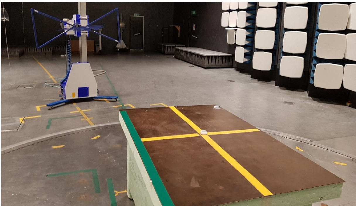
Test set up radiated emission 30 MHz – 1GHz
