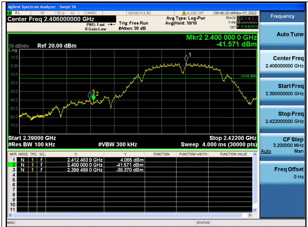
Test_Graph_802.11b_ANT1_2412_1Mbps_Lower Band Edge Emissions
