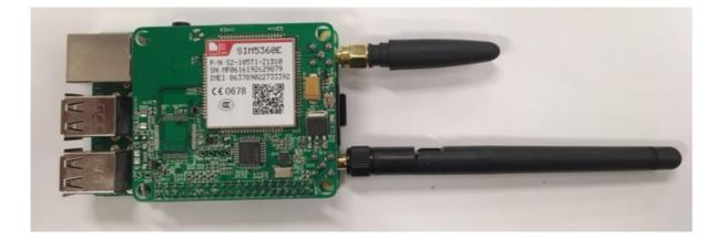
**Descriptions:** The hub is used to receive RF 433Mhz signals sent by other separate PIR sensors/devices – and thereafter transmit the data to 3G network via embedded 3G module (with 3G simcards)
