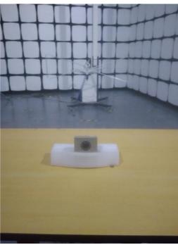
Radiated Emission test view (Frequency above 1GHz)
