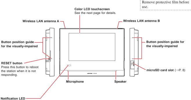
Indicates the current status of the station by lighting up or flashing.
