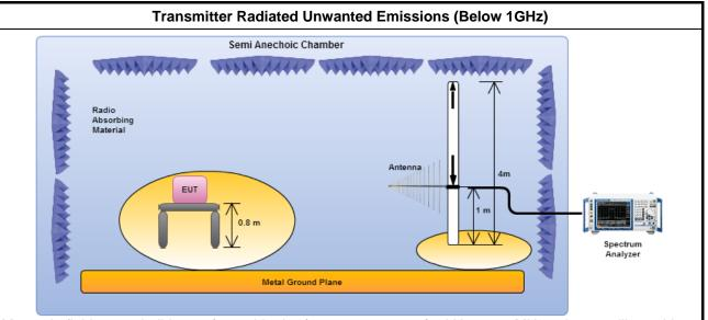
Magnetic field tests shall be performed in the frequency range of 9 kHz to 30 MHz using a calibrated loop antenna. Electric field tests shall be performed in the frequency range of 30 MHz to 1000 MHz using a calibrated bi-log antenna.
