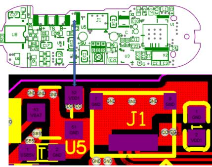
Changed to: U5, LRC6230, 3.3V regulator IC, package DFN1\*1-4. (New)
