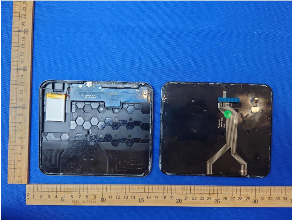
Internal View of EUT-1
