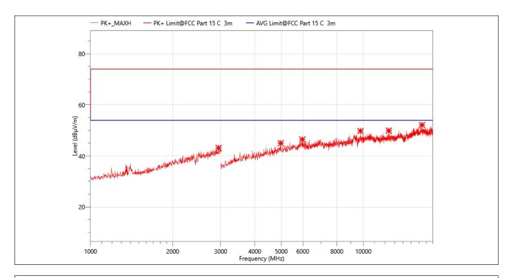
EUT: Temperature: **Portable Wireless Speaker** 24.5℃ M/N.: BTS13 **Humidity:** 55%RH **Power Rating:** Mode: 3-DH5 2441MHz **DC 3.7V Test Engineer: Test Time:** 2023-08-03 **Berny**
