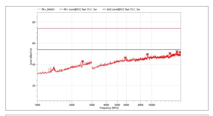
**EUT: Portable Wireless Speaker Temperature:** 24.5℃ M/N.: BTS13 **Humidity:** 55%RH Mode: 3-DH5 2480MHz **Power Rating: DC 3.7V Test Time:** 2023-08-03 **Test Engineer: Berny**
