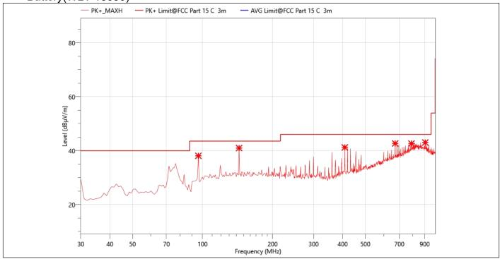
**EUT: Portable Wireless Speaker** Temperature: 24.5℃ M/N.: BTS13 **Humidity:** 55%RH Power Rating: 3-DH5 2402MHz **DC 3.7V** Mode: **Test Time:** 2023-08-03 **Test Engineer: Berny**
