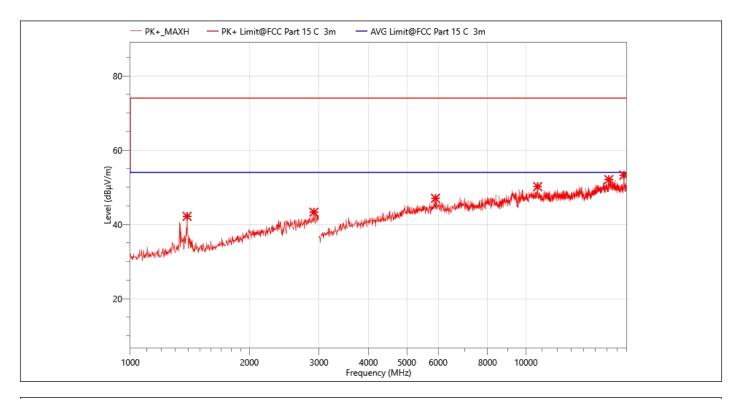
EUT: **Portable Wireless Speaker** Temperature: 24.5℃ M/N.: BTS13 **Humidity:** 55%RH Power Rating: Mode: 3-DH5 2402MHz **DC 3.7V Test Engineer: Test Time:** 2023-08-03 **Berny**
