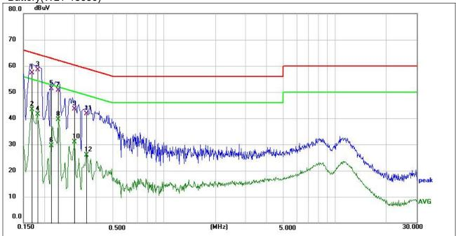
EUT: Portable Wireless Speaker Phase: L1 M/N.: BTS13 Temperature:  $26^{\circ}$ C Mode: 3-DH5 2402MHz Humidity: 54%RH
