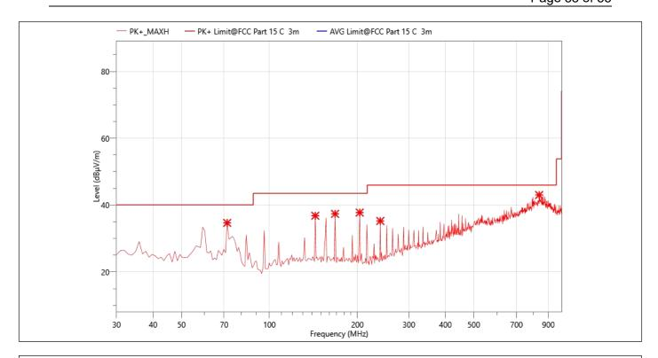
EUT: Portable Wireless Speaker Temperature: 24.5℃ M/N.: BTS13 **Humidity:** 55%RH 3-DH5 2402MHz Power Rating: DC 3.65V Mode: **Test Time:** 2023-08-03 **Test Engineer:** Berny
