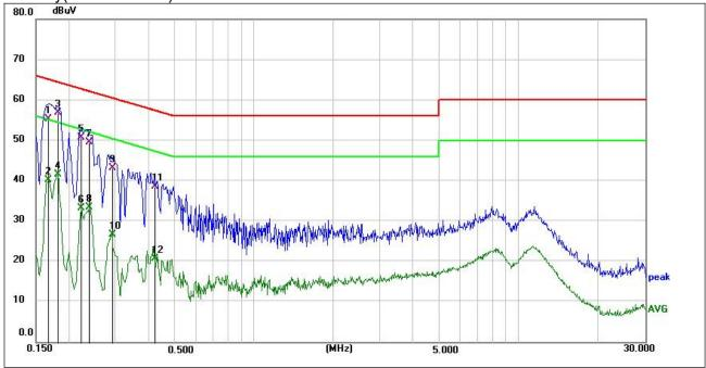
**EUT: Portable Wireless Speaker** Phase: L1 M/N.: BTS13 **Temperature:** 26℃ Mode: 3-DH5 2402MHz **Humidity:** 54%RH **Test Engineer:** Aiden **Power Rating:** AC120V/60Hz
