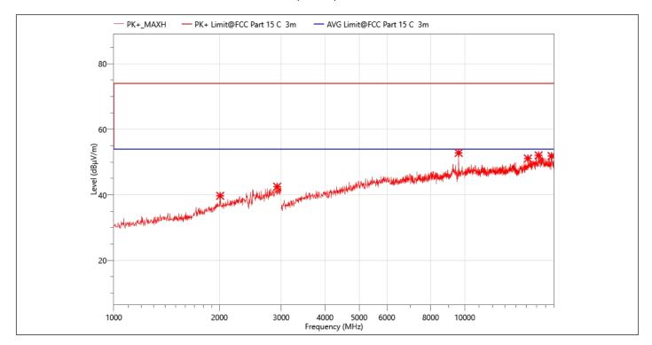
**EUT: Portable Wireless Speaker Temperature:** 24.5℃ M/N.: BTS13 **Humidity:** 55%RH Power Rating: Mode: 3-DH5 2402MHz **DC 3.7V Test Engineer:** Berny **Test Time:** 2023-08-03
