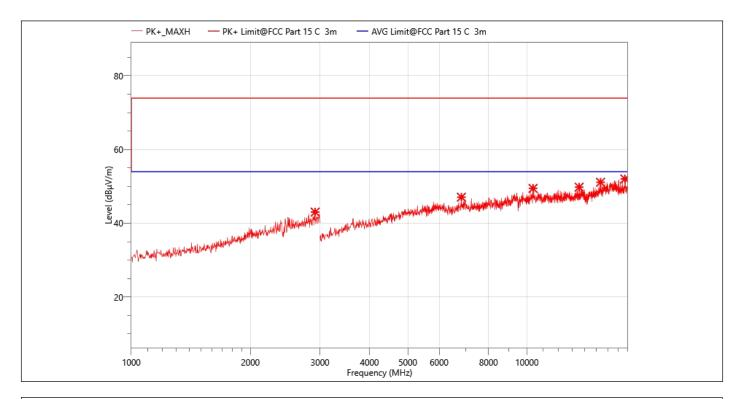
EUT: **Portable Wireless Speaker** Temperature: 24.5℃ M/N.: BTS13 **Humidity:** 55%RH Power Rating: Mode: 3-DH5 2441MHz **DC 3.7V Test Engineer: Test Time:** 2023-08-03 **Berny**
