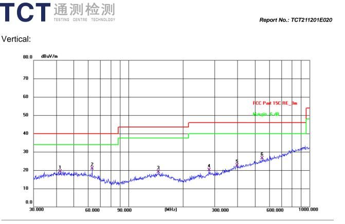
Polarization: Vertical Temperature: 25.2(C) Humidity: 55 % Site #2 3m Anechoic Chamber Limit: FCC Part 15C RE\_3m Power: DC 3.7 V Frequency Reading Factor Level Limit Margin Detector P/F No. Remark (dBuV) (dB/m) (dBuV/m) (dBuV/m) (MHz) (dB) 5.32 19.28 40.00 1 42.0066 13.96 -20.72 QP Ρ 63.0916 8.48 12.50 20.98 40.00 -19.02 QP Ρ 2 3 146.3735 5.82 13.30 19.12 43.50 -24.38 Ρ QP
