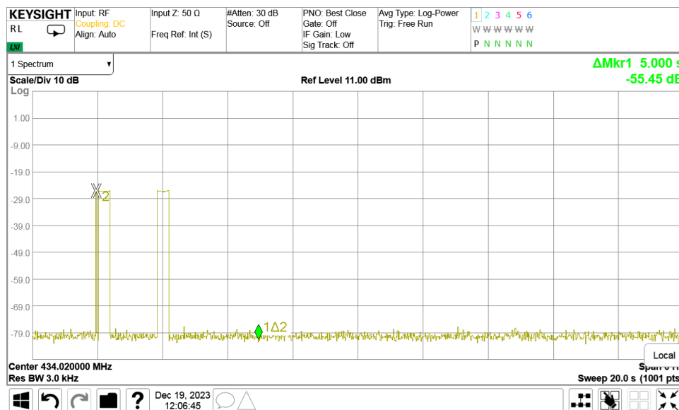
Plot 7.1.1 Transmitter shut down test result
