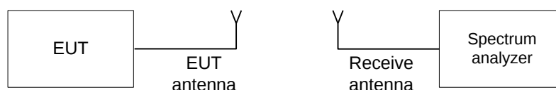
Figure 7.4.1 Occupied bandwidth test setup
