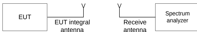
Figure 7.1.1 Setup for transmitter shut down test
