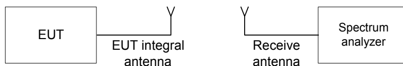
Figure 7.1.1 Setup for transmitter shut down test
