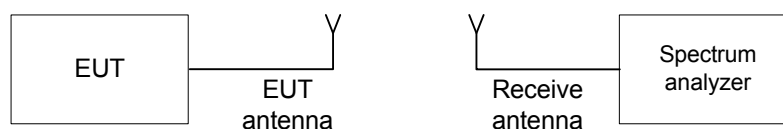
Figure 7.3.1 Occupied bandwidth test setup
