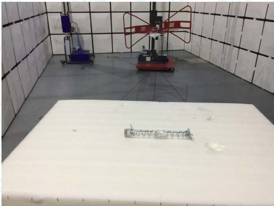
Photo of Setup for Radiated Emission (Below 1 GHz)-12 inch Antenna
