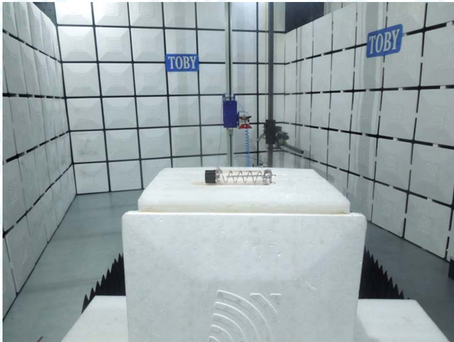
Photo of Setup for Radiated Emission (Below 1 GHz)-12 inch Antenna
