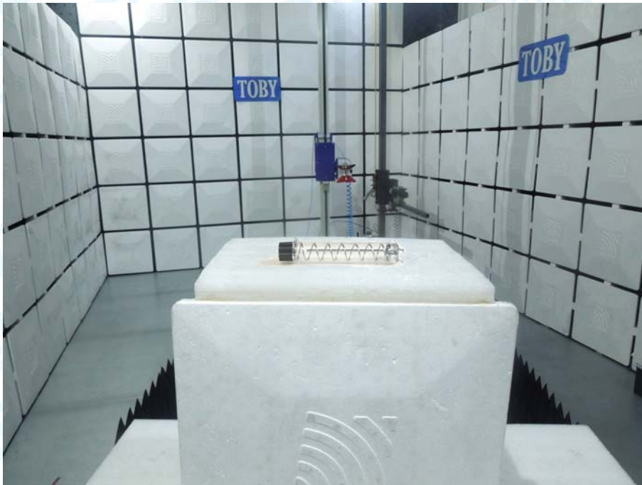
Photo of Setup for Radiated Emission (Above 1 GHz)-9 inch Antenna
