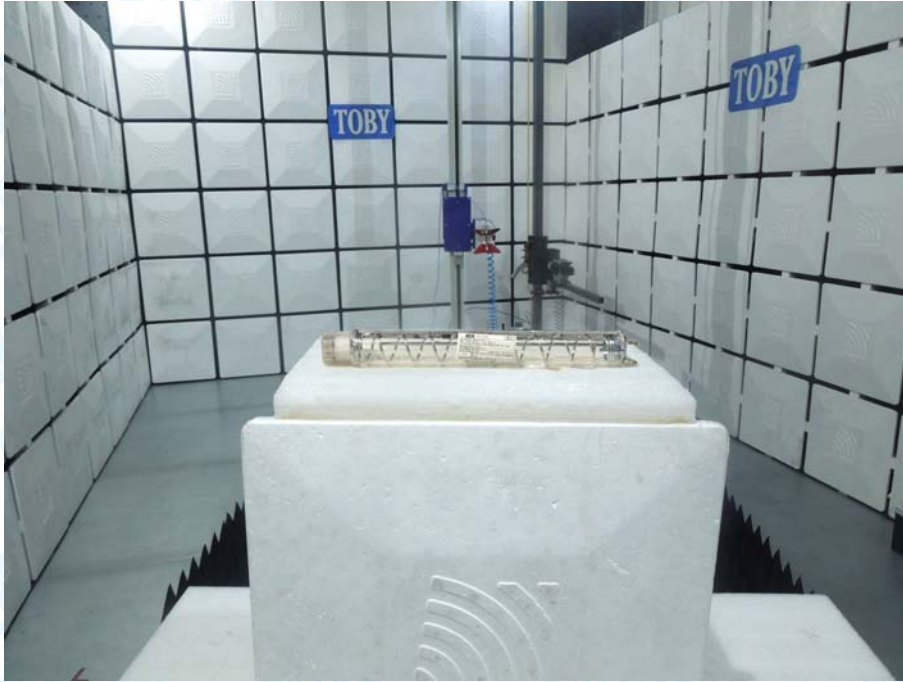
Photo of Setup for Radiated Emission (Above 1 GHz)-9 inch Antenna
