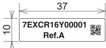
\*This label contains the serial number and the reference number for internal use.
