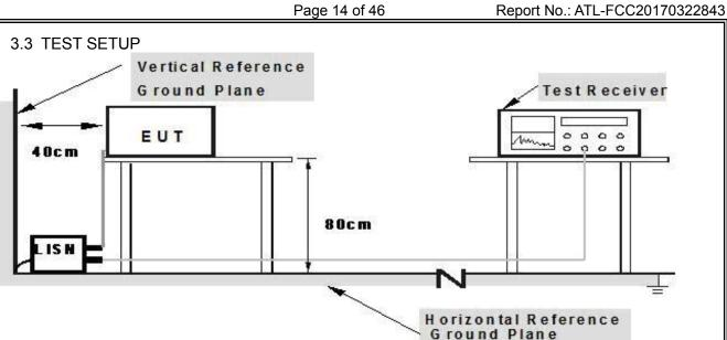
Note: 1. Support units were connected to second LISM. 2.Both of LISMs (AMM) are 80 cm from EUT and at least 80 from other units and other metal planes
