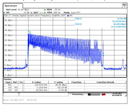
7.4.2. Transmitter Frequency Stability – Voltage 1 of 2 (-5% - 4.75 VDC, 20°C)
