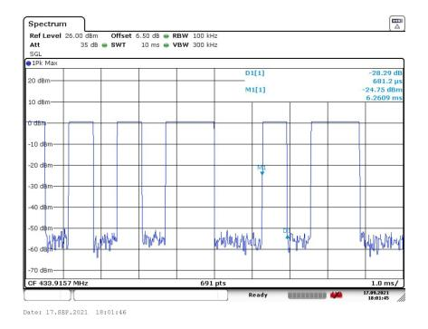
The graph shows the duration of 'on' signal. From Marker 1 to Delta 1, duration is 0.681ms.
