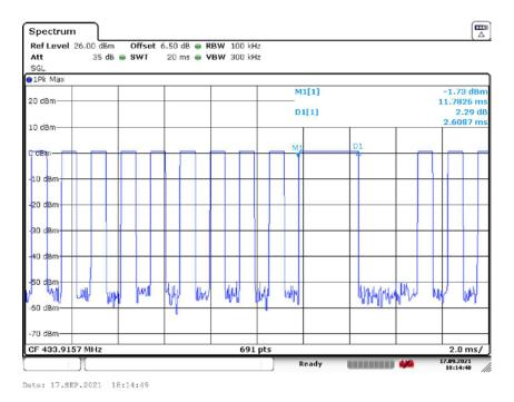
The graph shows the duration of 'on' signal. From Marker 1 to Delta 1, duration is 2.609ms.
