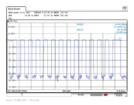
The graph shows the duration of 'on' signal. From Marker 1 to Delta 1, duration is 1.319ms.
