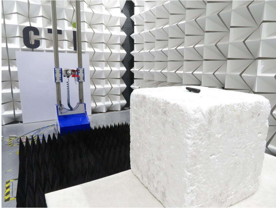
Radiated spurious emission Test Setup-3(Above 1GHz)
