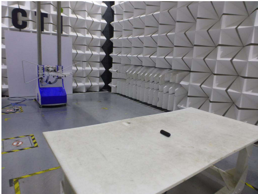
Radiated spurious emission Test Setup-1(30MHz-1GHz)
