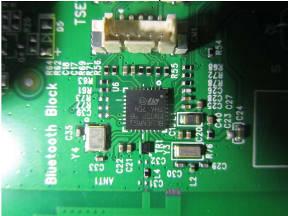
EUT – BT Chip View
