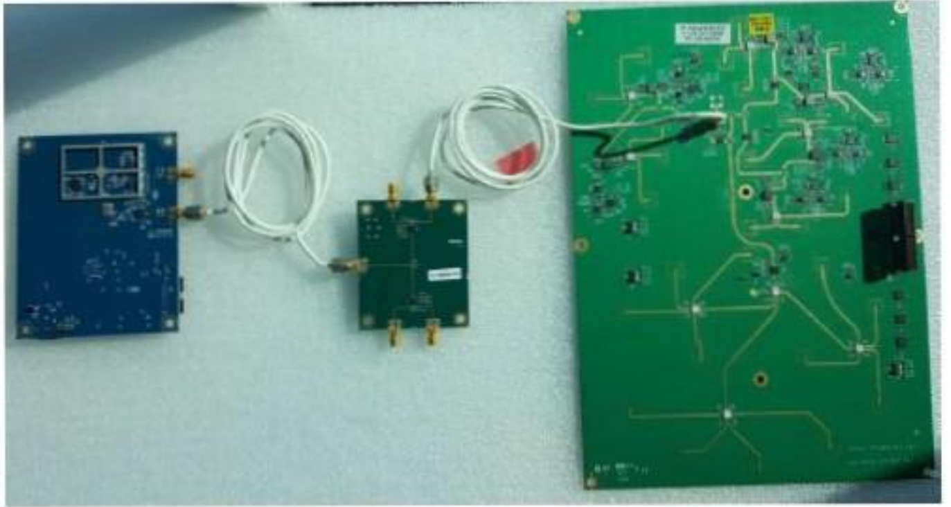
Figure 8. Photo, Local Oscillator to Transmitter
