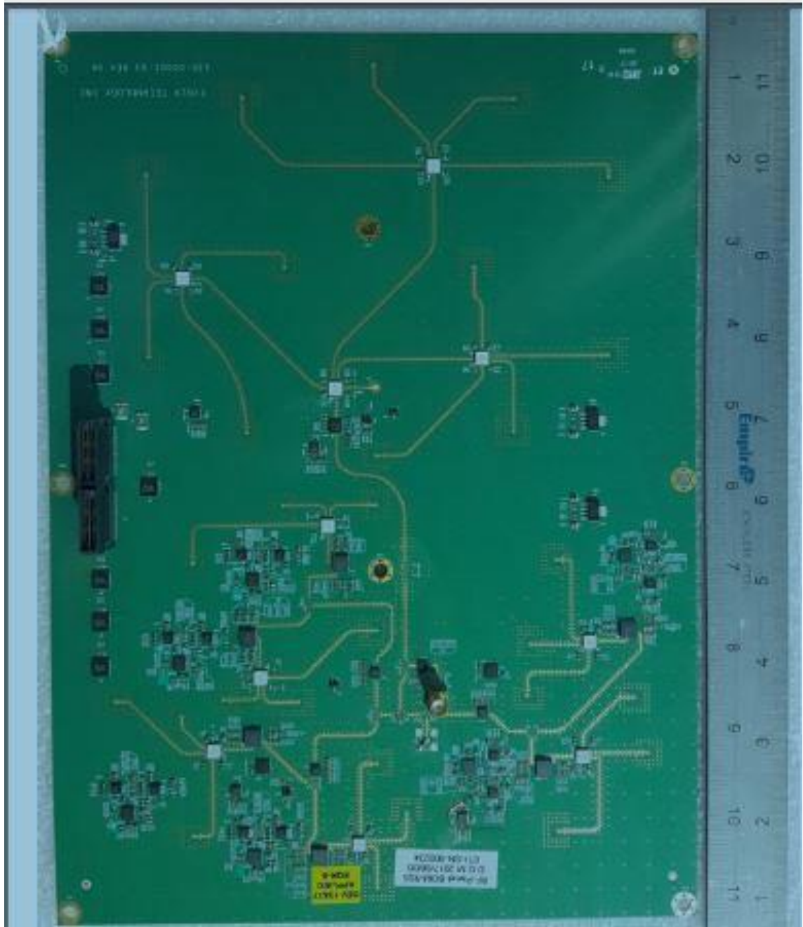
Figure 7-PCBA, RF Panel, Front (Component Side)
