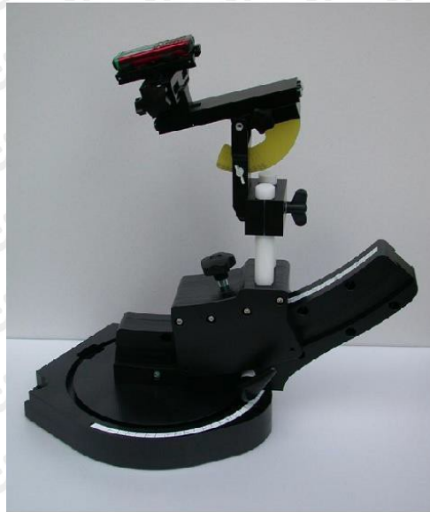
Device holder supplied by SPEAG
