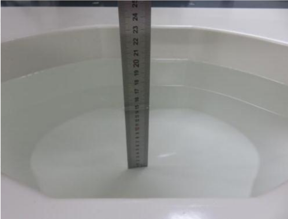
Photograph of the depth in the Head Phantom (2300MHz, 15.7cm depth)
