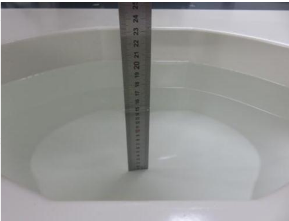
Photograph of the depth in the Head Phantom (2450MHz, 15.6cm depth)
