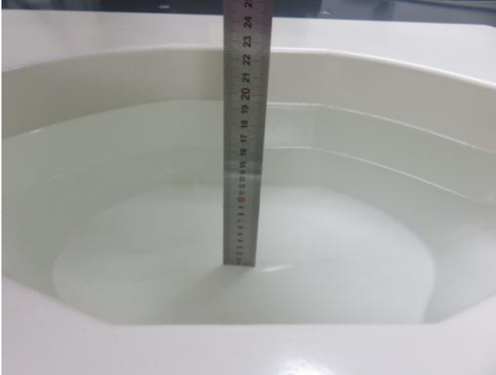
Photograph of the depth in the Head Phantom (835MHz, 16.1cm depth)
