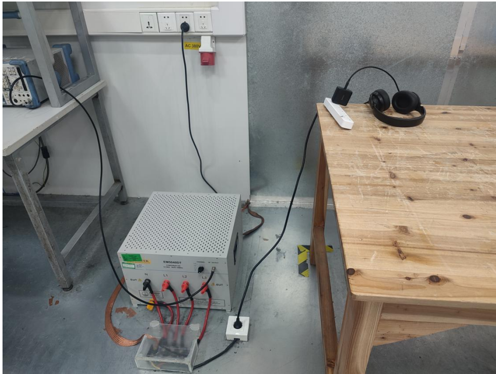
Photo of Conducted Emission Measurement
