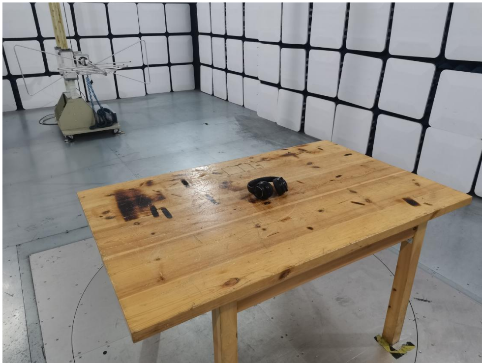
Photo of Radiation Emission Test
