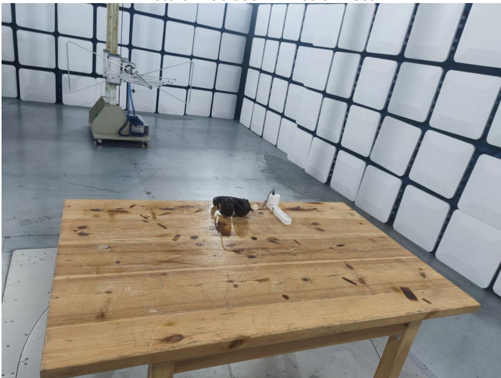
Photo of Radiation Emission Test
