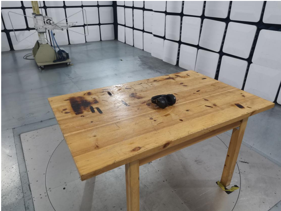
Photo of Radiation Emission Test
