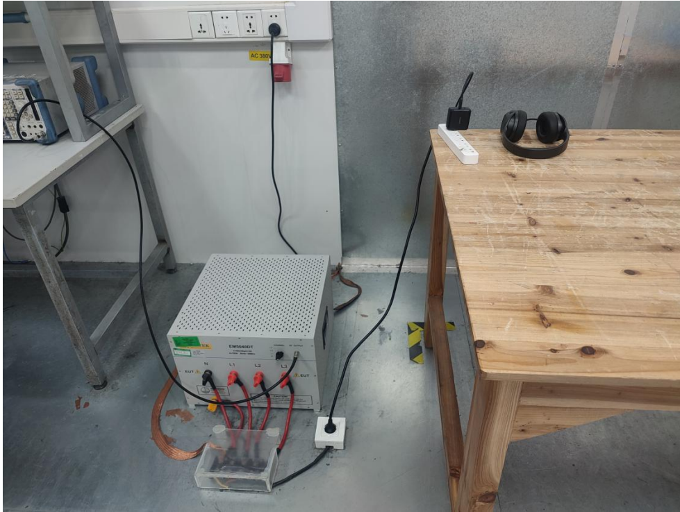
Photo of Conducted Emission Measurement
