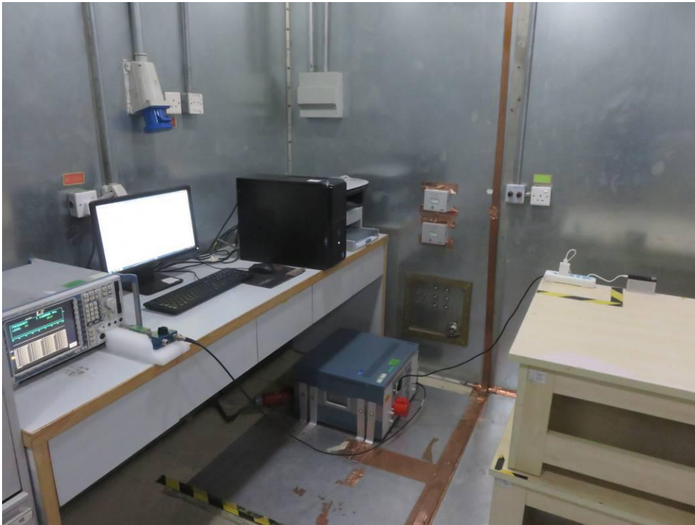
FCC RADIATED EMISSION TEST SETUP
