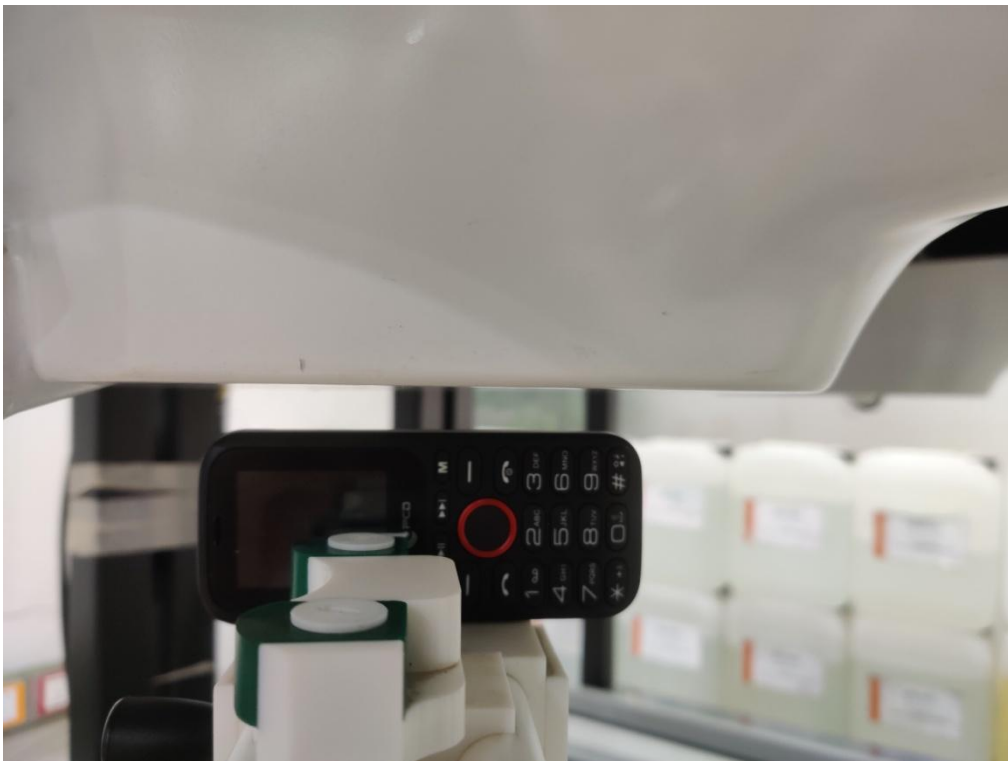
Body right side(separation distance is 10mm)
