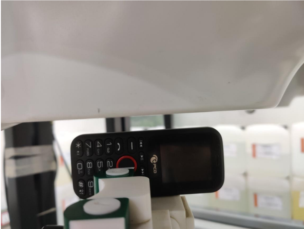
Body left side(separation distance is 10mm)
