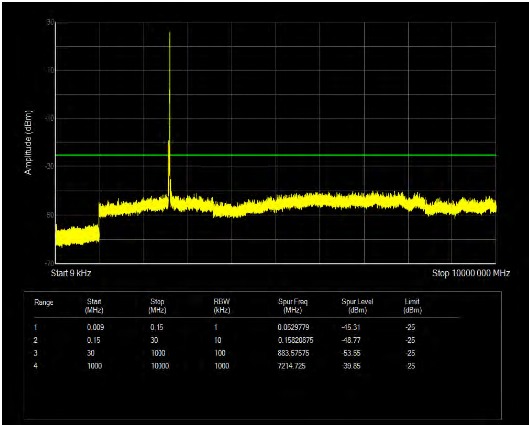
Band41(2555-2655) QPSK BW=20MHz Channel=40740 RB Size=1 Position=#Max
