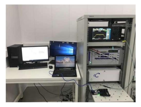
1.2 Set-up for Spurious Emissions below 1GHz
