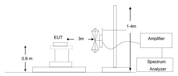
RADIATED EMISSION TEST SETUP ABOVE 1000MHz
