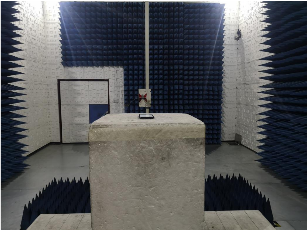
RADIATED EMISSION TEST SETUP ABOVE 1GHZ
