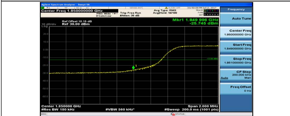
Channel Bandwidth: 10 MHz_LCH_16QAM_50RB#0
