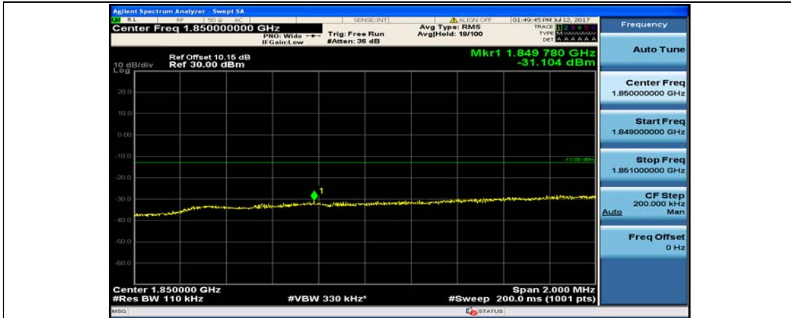
Channel Bandwidth: 10 MHz_LCH_16QAM_25RB#25
