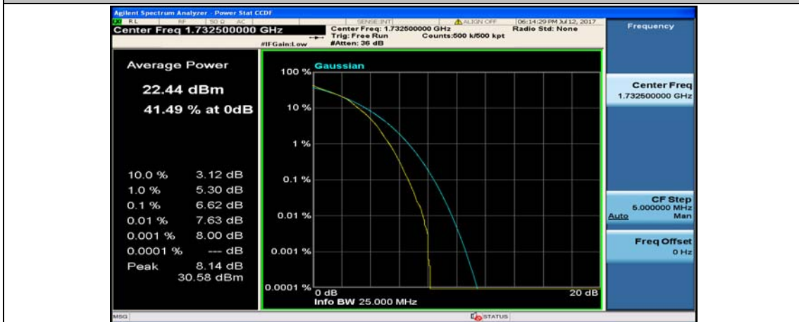
(Channel Bandwidth:15 MHz)_MCH_16QAM_37RB#38
