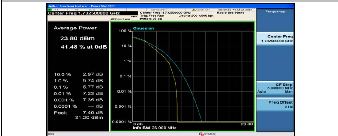
Channel Bandwidth: 10 MHz_MCH_16QAM_1RB#24
