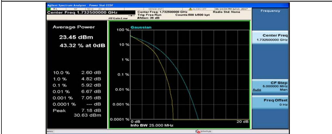
(Channel Bandwidth:15 MHz)_MCH_QPSK_37RB#18
