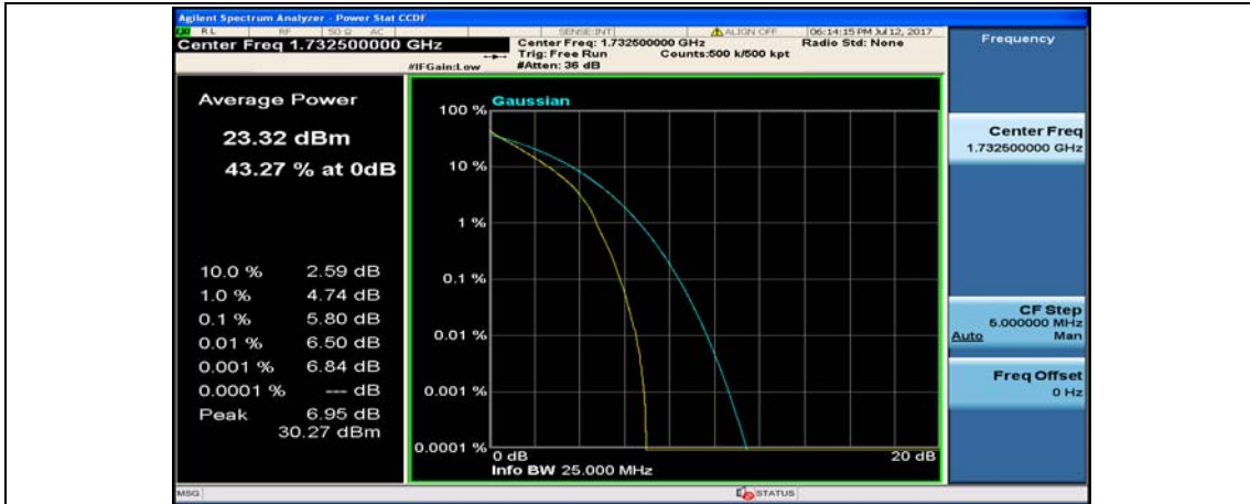
(Channel Bandwidth:15 MHz)_MCH_QPSK_75RB#0
