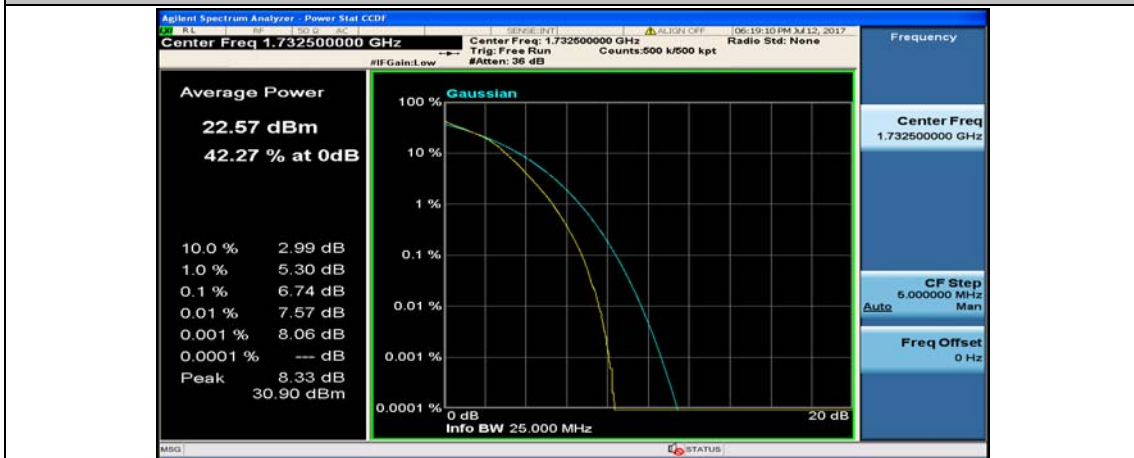
(Channel Bandwidth:20 MHz)_MCH_16QAM_50RB#25
