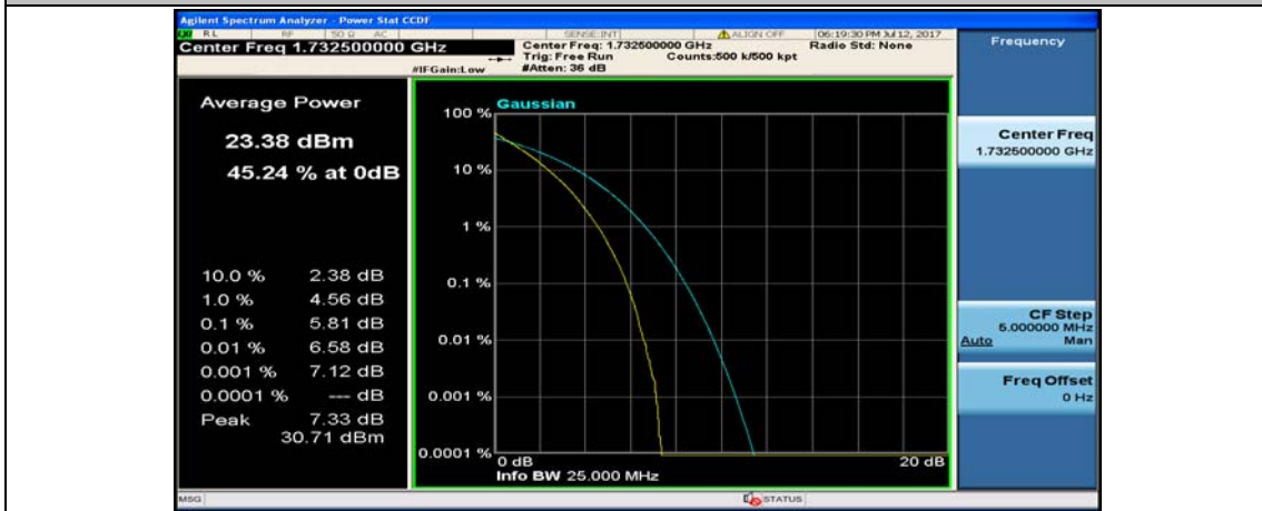
(Channel Bandwidth:20 MHz)_MCH_QPSK_100RB#0
