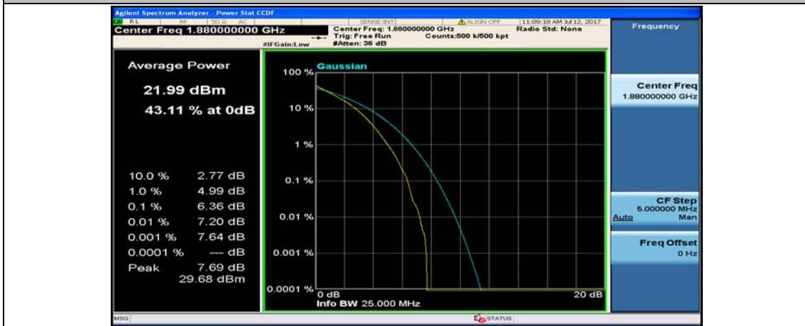
(Channel Bandwidth: 1.4 MHz)_MCH_QPSK_6RB#0
