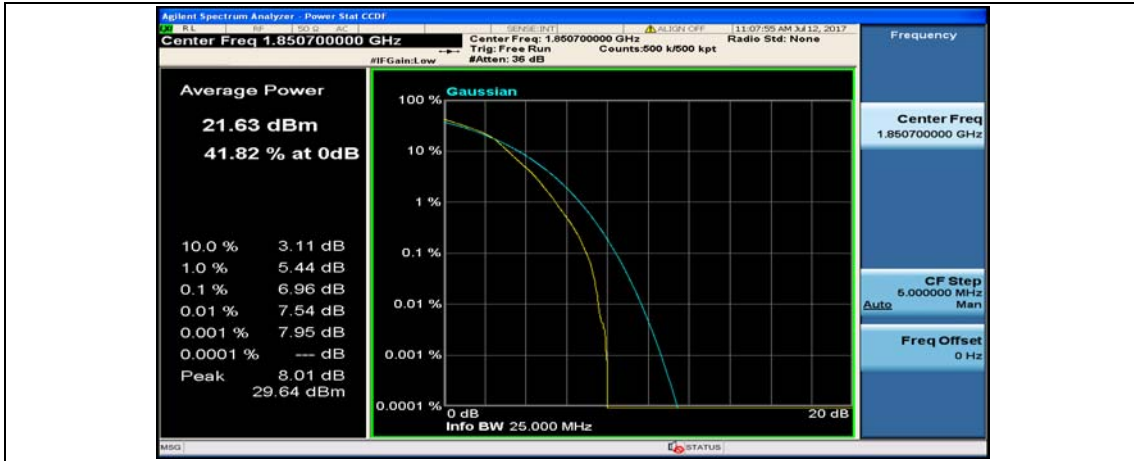
(Channel Bandwidth: 1.4 MHz)_MCH_16QAM_1RB#0
