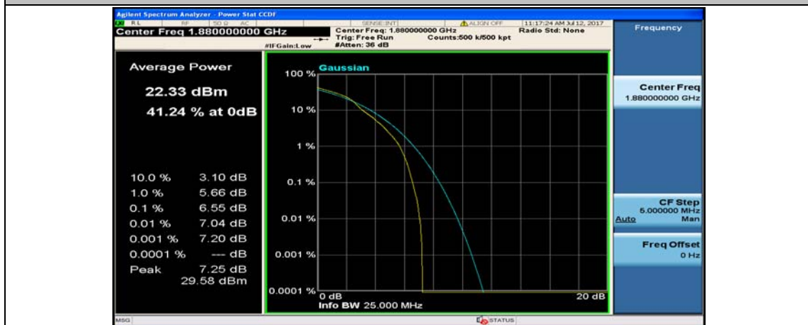
(Channel Bandwidth: 5 MHz)_MCH_16QAM_1RB#12
