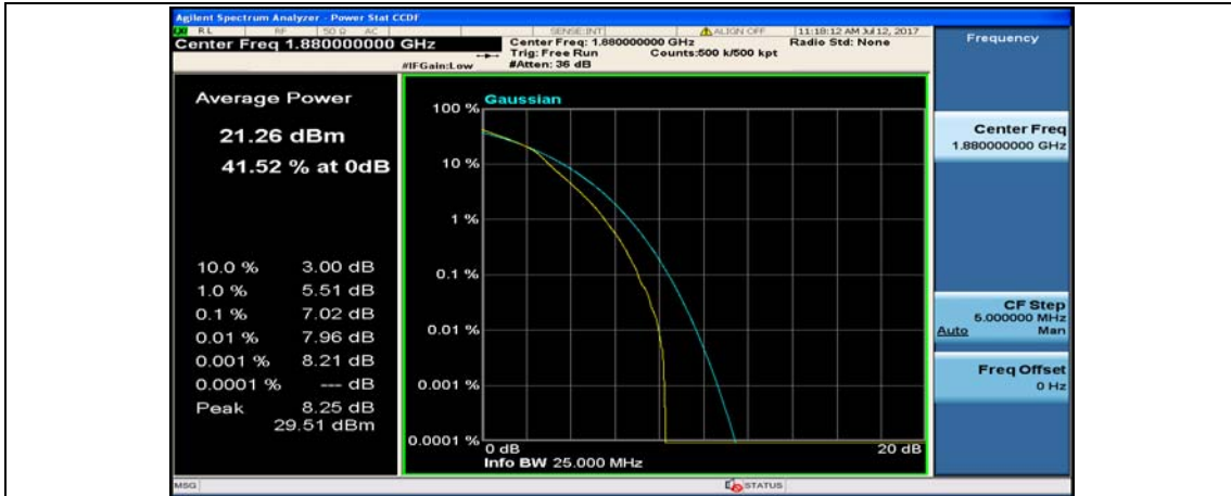
(Channel Bandwidth: 5 MHz)_MCH_16QAM_25RB#0
