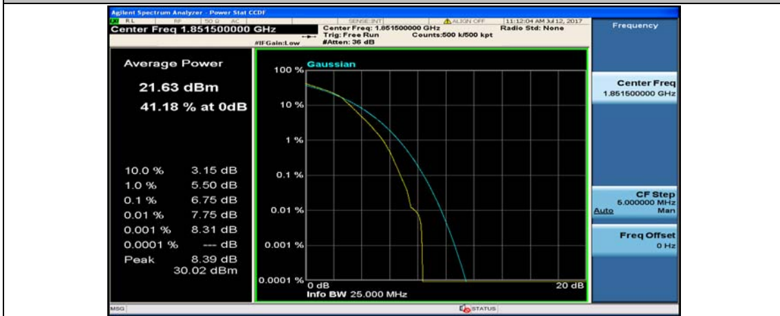
(Channel Bandwidth: 3 MHz)_LCH_16QAM_8RB#7
