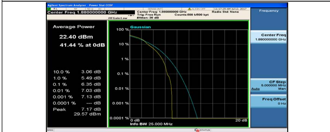
(Channel Bandwidth: 5 MHz)_MCH_16QAM_1RB#24
