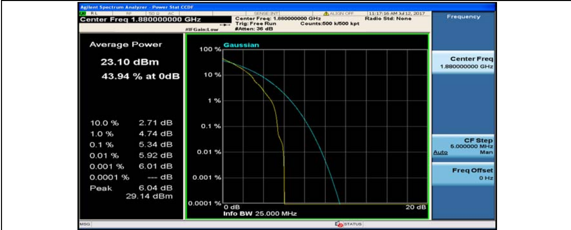
(Channel Bandwidth: 5 MHz)_MCH_QPSK_12RB#0
