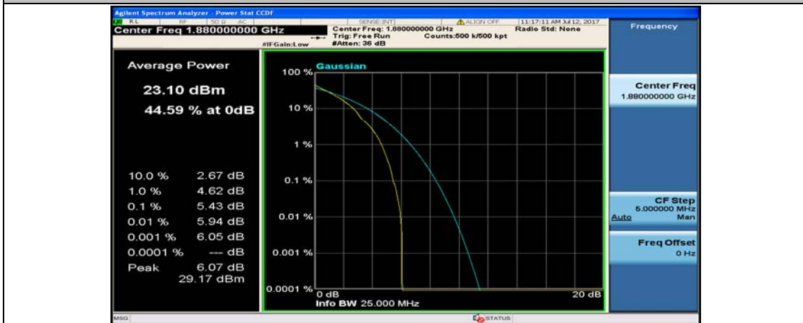
(Channel Bandwidth: 5 MHz)_MCH_QPSK_1RB#24
