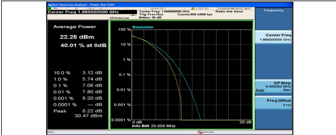
(Channel Bandwidth: 1.4 MHz)_MCH_16QAM_6RB#0
