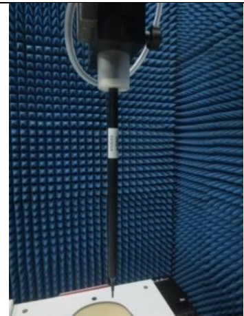
Fig.8.2 Photo of E-Field Probe
