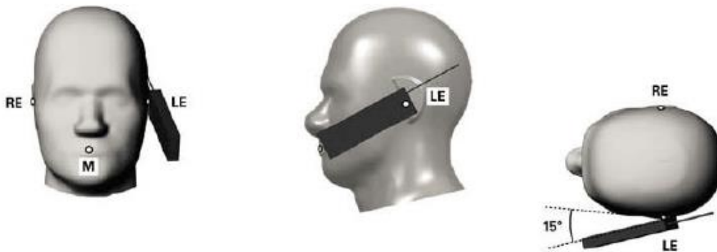
Fig.11.4 Illustration for Tilted Position
