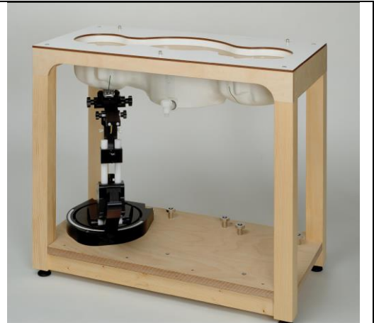
Fig. 8.7 Photo of SAM Twin Phantom
