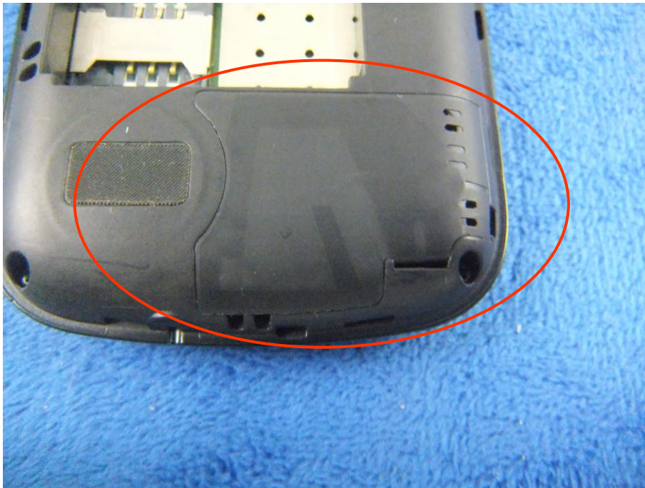
GSM/WCDMA - Antenna View
