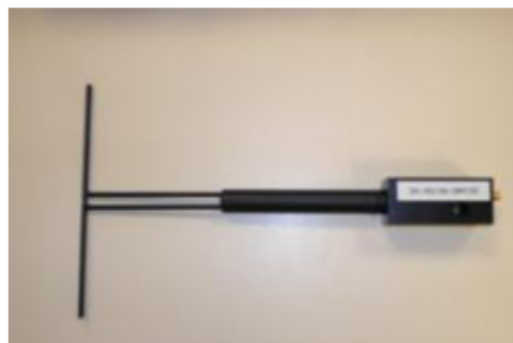
Figure 1 – Satimo COMOSAR Validation Dipole
