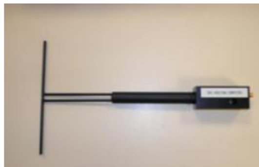
Figure 1 – Satimo COMOSAR Validation Dipole
